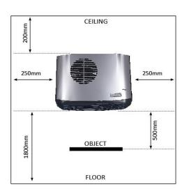
**Important:** The heater must NOT be located immediately below a socket outlet or within reach of a bath or shower.
