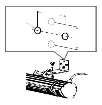
**Figure 3:** Mounting bracket (wall bracket) and raw plugs provided. Connection from the wall to Fresco.
