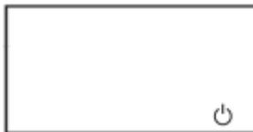
When the screen is switched off, the first time any key is pushed the screen lights up without activating the function controlled by the key pushed.
